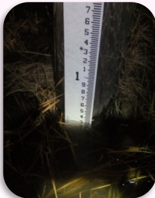
Tide staff at installation and during flood event, surveyed to vertical reference frame.
