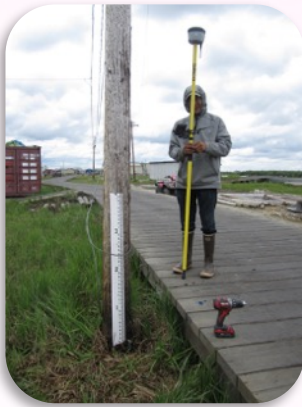
Tide staff at installation and during flood event, surveyed to vertical reference frame.
